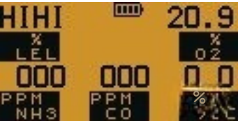
Display in alarm conditions
